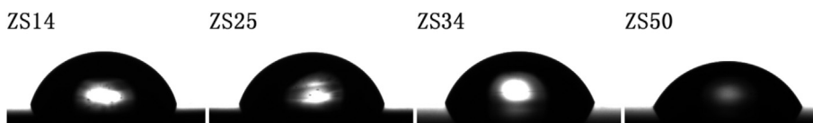
Fig. 10. Pictures of water drops on the four ZS membranes in the water contact angle measurement.
